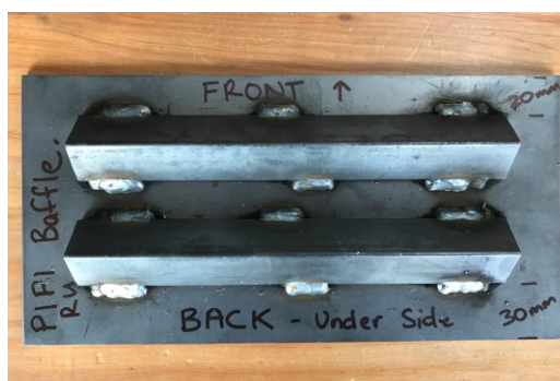
Baffle showing underside. Smooth surface faces up into fire. Back fitted hard to rear of fire box. 20mm gap at front edge. 30mm gap at rear edge
